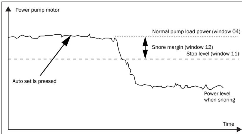
Fig. 2 Auto set performed at normal pumping
