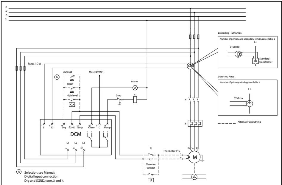
Fig. 13 Single-pump system installation example (alternatively see Chapter 13).
