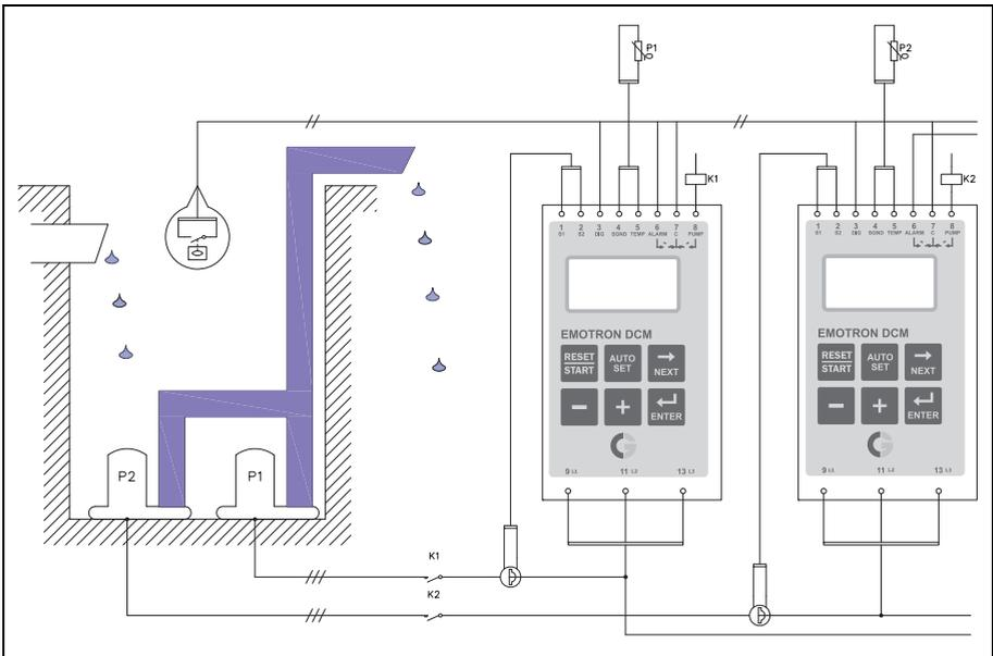
Fig. 15 Dual-pump application
