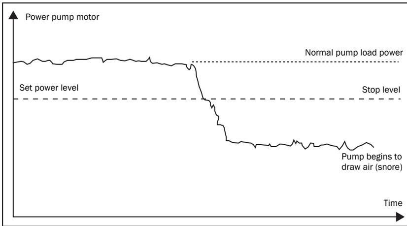
*Fig. 1 Pump operation*
