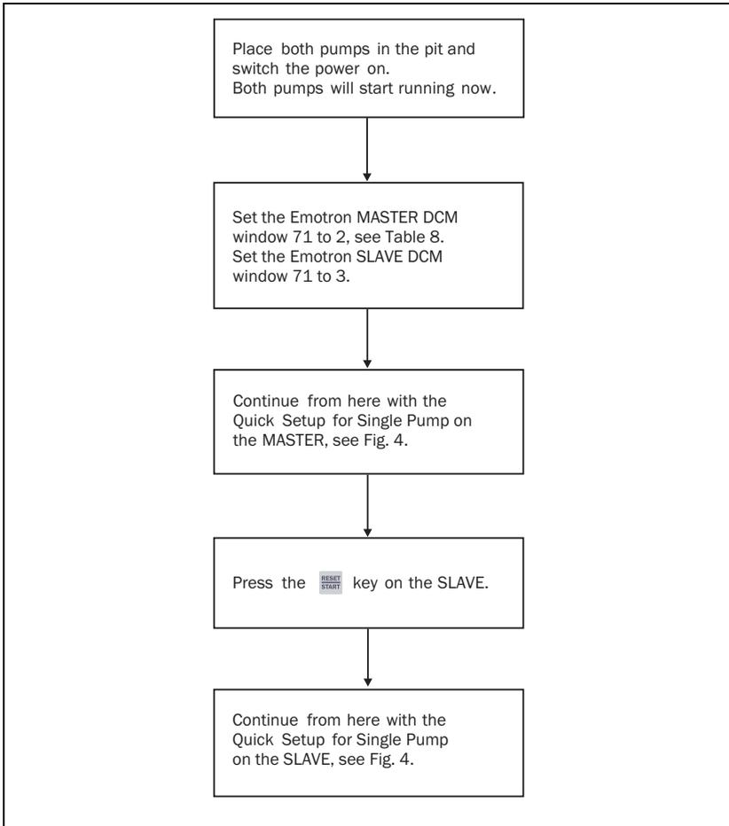
*Fig. 5 Quick setup for dual-pump system (the pumps will start and stop during setup).*
