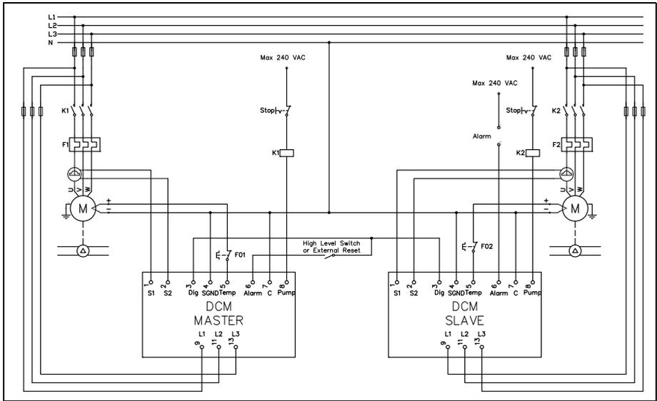
Fig. 16 Dual-pump example (alternatively, see the Appendix, Chapter 13)
