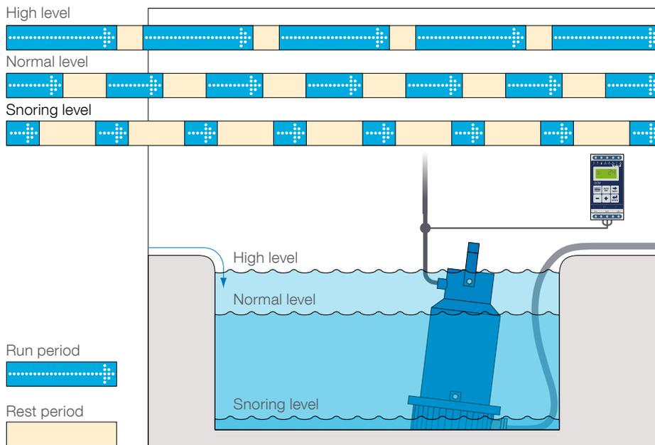
Different water levels for starting the pump can be entered via the control panel. The Emotron DCM then uses an algorithm to calculate the appropriate run and rest periods. Pump operation is automatically adapted to the pit filling rate, minimizing energy consumption and component wear.
