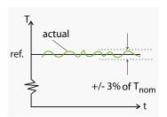
Open loop = <3 % for speeds 10 - 100% of rated, and <10% at zero speed (% of  $n_{nom}$ ).
