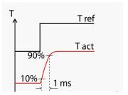
Open loop: = 100 % torque step rise time = 1 ms.
